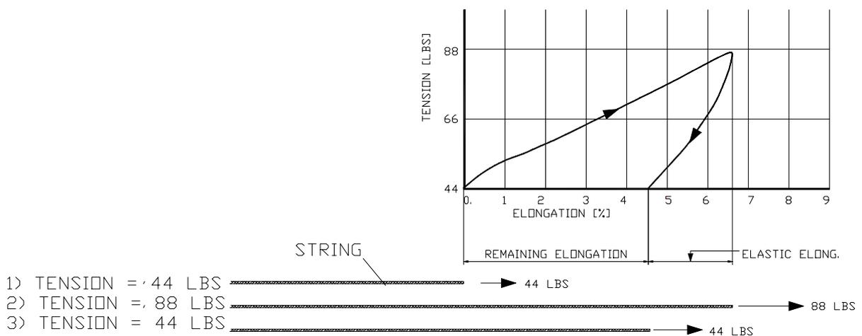
The figure shows the principle of measuring the elongation of a string.
